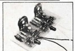
A fool-proof electronically controlled battery charger with current and voltage regulation, auto taper charging, short circuit and reverse polarity protection and LED indication of operation.
