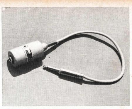
Mumetal-shielded microphone matching transformer, made by Grampian.
