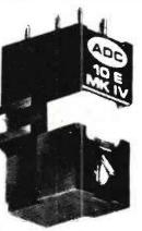
ADC 10E mk4 .... \$45.00 Type: Induced Magnet\* Output: 4 mV at 5.5 cms/ sec. recorded velocity Tracking Force: 7 gram Frequency Response: 10 Hz to 20 kHz ± 2 dB Channel Separation: 30 dB from 50 Hz to 12kHz Compliance: 35 x 10 ° cms / dyne Elliptical Stylus Tip: Contact radius: .0003"; lateral radius: .0007" IM Distortion: Less than  $\frac{1}{2}$ "% - 400 & 4000 Hz at 14.3 cms / sec. recorded velocity Vertical Tracking Angle: 15 degrees Recommended Load Impedance: 47000 ohms nominal
